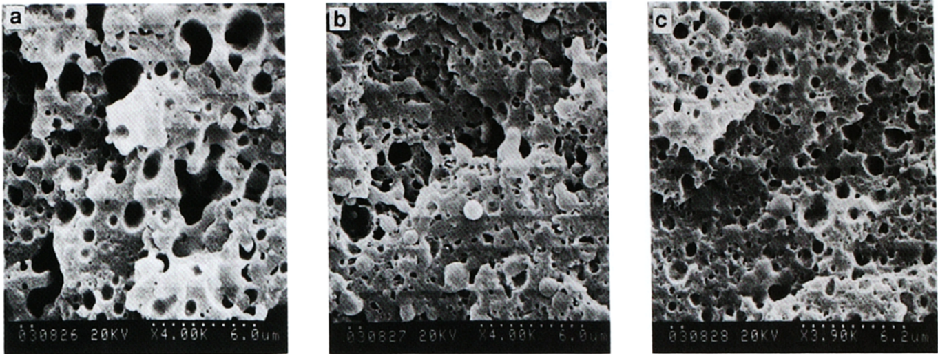
Figure 4 SEM micrographs of the blends: (a) PBT/ABS/SAG0/ETPB = 75/25/5/0.01; (b) PBT/ABS/SAG2/ETPB = 75/25/5/0.01; (c) PBT/ABS/SAG4/ETPB = 75/25/5/0.01
